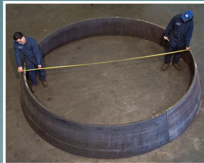
1-3/4" plate cone segments with a 151" minor diameter and a 169" major diameter in 90 degree segments
