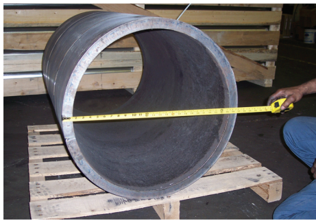
1-1/2" plate 45" long rolled to a 24" inside diameter
