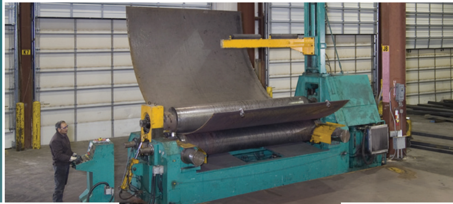
2" x 12' plate roll can roll 30' lengths
